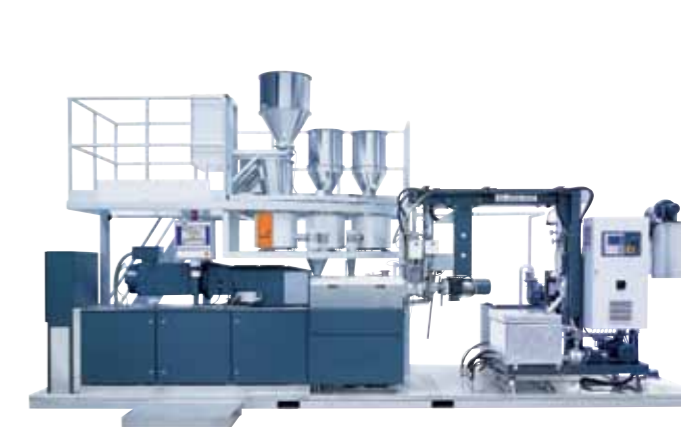
C-FLEX M installed on a co-rotating twin-screw extruder
