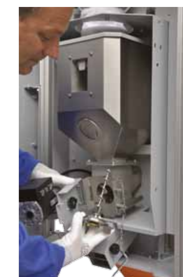
One-sided bearing mounted dosing screw with a quick release connection
