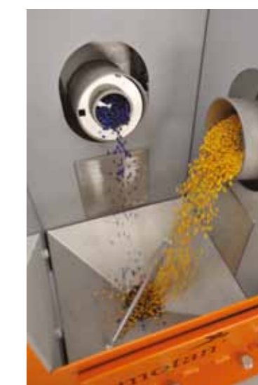
Gravity mixing principle
